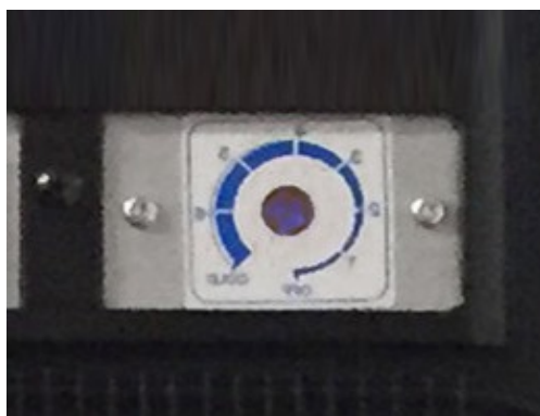
Photo detail rear thermostat
