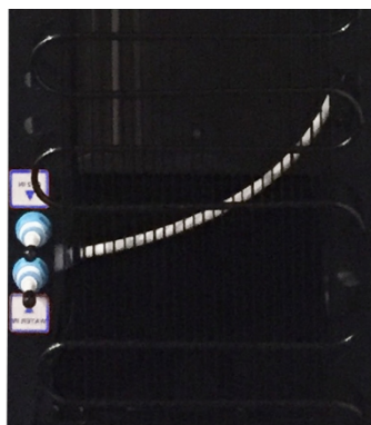
CO2 inlet detail HIGH quick coupling, WATER inlet LOW quick coupling
