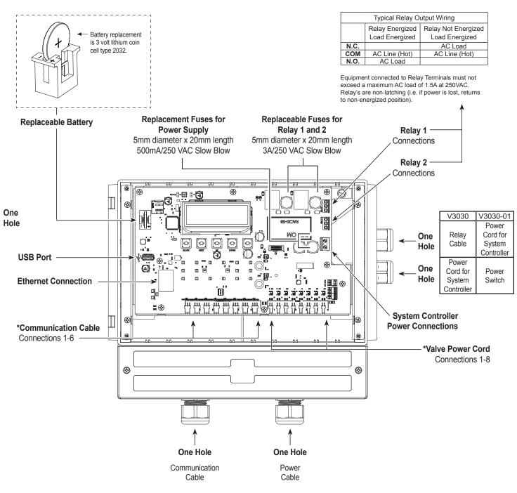
\*Use Communication Cable and Power Cord Connections in consecutive ascending order, starting with 1. \*\*If using Ethernet Cable drill hole and use. V4096 SC ETHERNET ADAPTER to provide strain relief.
